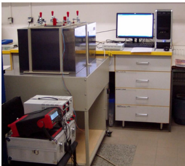
Fig. 1 The isothermal heat flow calorimeter for large-volume applications
